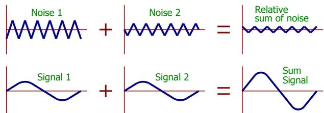
With the new way in the QAmpI of combining many small amplifiers a reduction in the noise level by 85% is possible, in comparison with conventional solutions.
